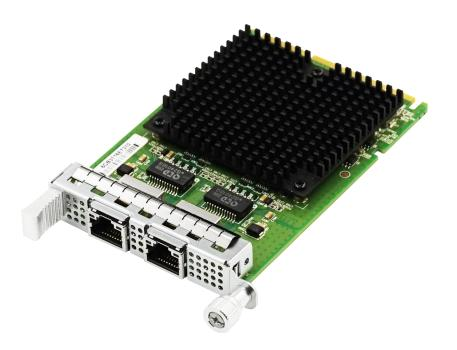
LRES3041PT-OCP is an OCP3.0 SFF dual-port copper Gigabit Ethernet network adapter independently developed by Shenzhen Lianrui Electronics Co., Ltd. based on the Intel I350 master control solution. This adapter is mainly designed for use in servers and their application equipment.
